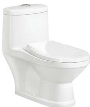
115010271 ACL VW10310 Children Wash Down One Piece WC Suite 4.5L (Single) Top Push Button, PP Seat Cover S Trap: 200mm Size: 520 x 280 x 525 (mm)
